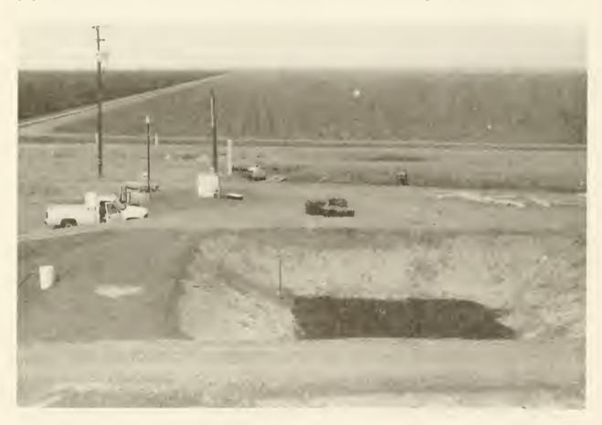
Panoche Water District is testing the removal of selenium by passing drainage water through a bed of iron filings in the bottom of this basin.
